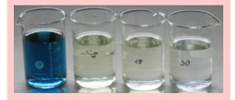
Very powerful oxidising agent Hydroxyl radicals are generated on the surface of the anodes which reacts with organics and oxidises them completely and coverts to carbon Dioxide. The entire process is handled automatically.
